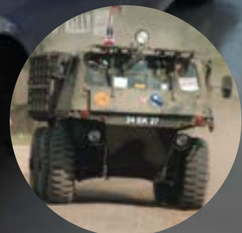
The Alvis Stalwart amphibian cargo carrier vehicle as used by British forces in the late '60s and into the early '80s
