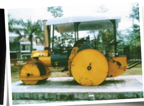
▲ A later Albaret of the smaller 'DN Type' (6 to 8 tonnes) at Purwokerto, Central Java. This is No.2120 of 1954. Andi Slender
